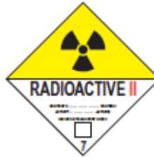
Category II-YELLOW Does not exceed 500 µSv/h at any location on the external surface of the package and the transport index does not exceed 1.
