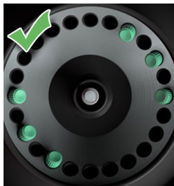
A) Rotor properly balanced
