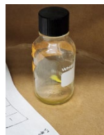
Figure 1. A waste bottle suspected to contain unstable PEROXIDES should be considered extremely dangerous
