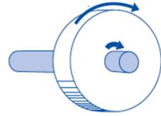
Wheel and axles are used to help move heavy objects more easily
