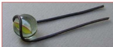
4. Tape the wire to the bottom of the mirror prism, trying to keep the marble covering the hole for the best effect.
