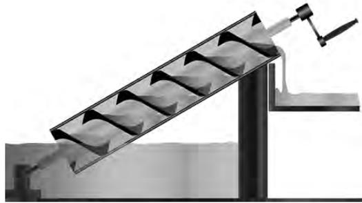
Figure 1: Inside view of Archimedes screw pump. (<http://empoweringpumps.com/screw-pump-basics/>)
