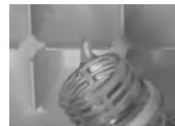
3. Place each nail into one well of vinegar and make sure the copper wire is bent so that it goes into the vinegar in the next well. There should be only vinegar between the metals in each well.
