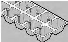
4. Place one wire of the LED into a well with only copper wire inside. Place the other wire into a well with only a nail in it. If LED doesn't light up, turn LED around so that wire goes in the other well because LEDs are one-way streets for current.
