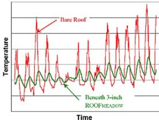
**Figure 9: Temperature comparison with and without green roof<sup>34</sup>**
