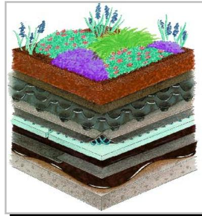
**Example:** Consider the above depicting an Intensive Garden Roof Assembly with 8" of soil. The dry weight of the assembly would be approximately 50 LB. / S.F. The wet weight (saturated weight) of the assembly would be approximately 78 LB. / S.F. One inch of water weighs 5.2 LB. The difference between the two is 28 LB., so the equivalent of over 5 inches of rain would have to fall to saturate the assembly!
