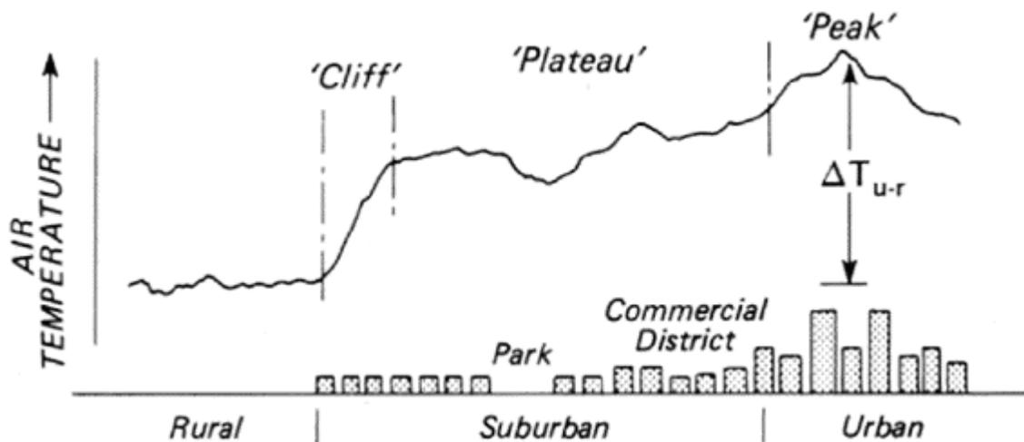
Figure 7. Generalized cross-section of an urban heat island<sup>1</sup>
