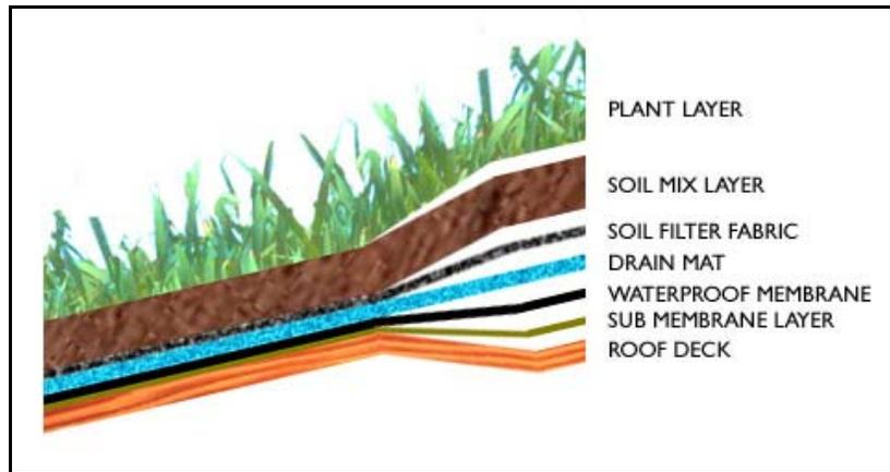
Figure 13. Green roof cross-section<sup>29</sup>
