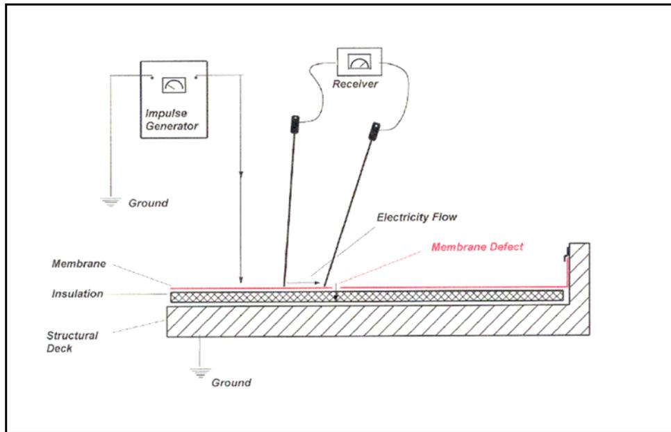
**Figure 14. Electric Field Vector Mapping Technology** <sup>38</sup>
